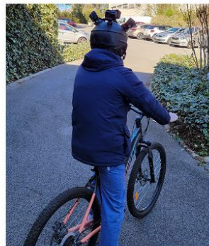
Fig. 9. Left: Our 6-GoPro HERO6 camera helmet rig. Middle: We performed captures on foot and (Right) on a bicycle at 6–7 km/h.
