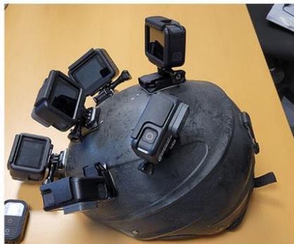
Fig. 9. Left: Our 6-GoPro HERO6 camera helmet rig. Middle: We performed captures on foot and (Right) on a bicycle at 6–7 km/h.
