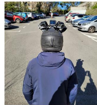
Fig. 9. Left: Our 6-GoPro HERO6 camera helmet rig. Middle: We performed captures on foot and (Right) on a bicycle at 6–7 km/h.
